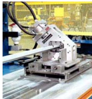
Figure 4. A self-contained style die is simple to changeover and good for open-loop measuring.
