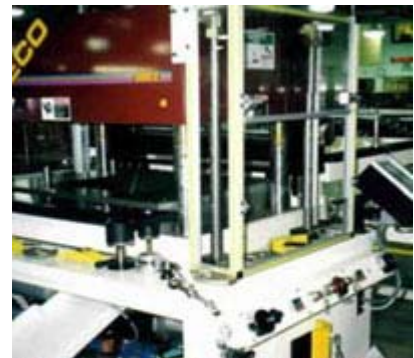
Figure 1. Without using a positive stop or some type of accelerator system, hydraulics don't make much sense in roll forming.
