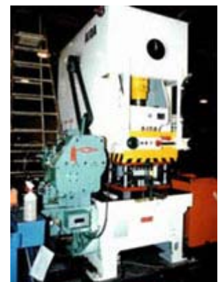
Figure 10. An OBI / OBS press easily slides a stationary die or a flying die in-and-out the entry or exit side.
