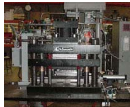
Figure 7. A fixed press with a die flying inside can mimic an air or mechanical press on an adjustable bed.
