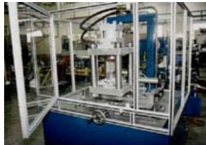
Figure 6. The fast changeover of a flying fixed press with a die inside makes it ideal when using multiple dies.
