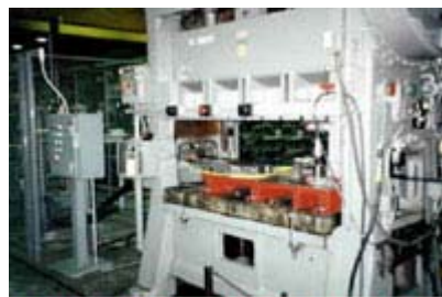
Figure 9. The large, stable ram on a straight side press reduces concern about the frame flexing.
